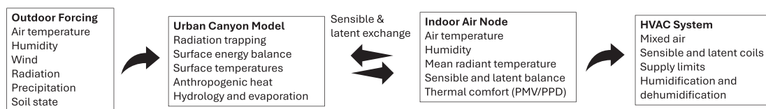
Fig. 2. Conceptual schematic of VCWG v3.1.0 illustrating two-way coupling between outdoor forcing variables, the urban canyon model, the indoor air node, and the HVAC system.
